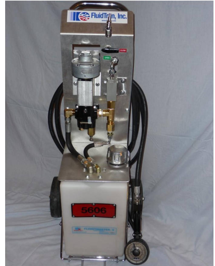
Landing Gear Servicing Unit (Liebherr/Embraer)
